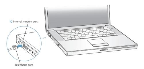
Make sure you connect the internal modem to an analog phone line—the kind used typically in homes. The modem will not work with a digital phone line.
